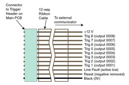
The function of the trigger outputs can be programmed as outputs 0001 to 0008 in menu 53.
